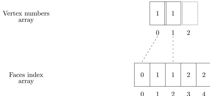
This example, in which the right-side elements (i.e. the triangles) belong to no specified group illustrates how elements with no associated data are handled: their index and that of the following element is simply the same.
